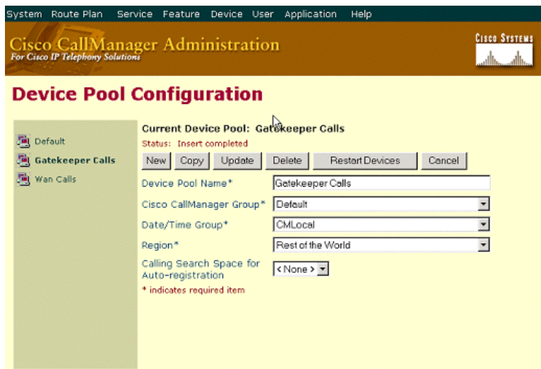
Figure 6-12 Configuring a Device Pool in Cisco CallManager
